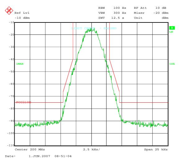
Figure 3 CMX7031/CMX7041 4.8kbps 4FSK I/Q Modulator RF Spectrum vs. Mask E
